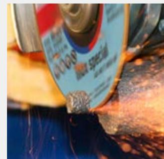
Deburr or grind immediately without changing discs.
