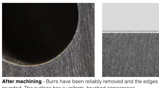
**After machining** - Burrs have been reliably removed and the edges rounded. The surface has a uniform, brushed appearance.
