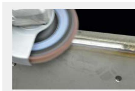
Removal of welding seams and attractive finish in a single process
