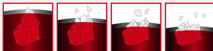
The new bond technology and the micro-crystalline structure of the ceramic grain ensure that new, extremely sharp cutting edges are continually released in a targeted manner. This guarantees that the CeraMaxx cutting and grinding discs can always put in a top performance – from start to finish. For maximum cutting speed, removal rates and service life.
