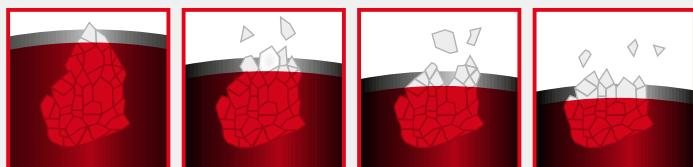
The new bond technology and the micro-crystalline structure of the ceramic grain ensure that new, extremely sharp cutting edges are continually released in a targeted manner. This guarantees that the CeraMaxx cutting and grinding discs can always put in a top performance – from start to finish. For maximum cutting speed, removal rates and service life.
