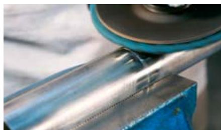
Sanding fine welding seams and removing thermal discolouration
