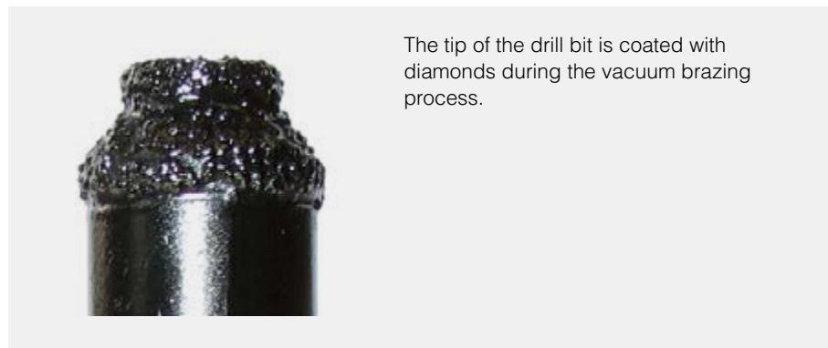
The tip of the drill bit is coated with diamonds during the vacuum brazing process.
