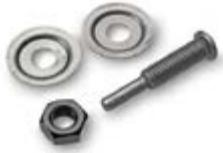
Tapered shank for power drill or ductile shaft for clamping polishing and satin finishing buffs with bore 10 mm, to diameter 100 mm.
